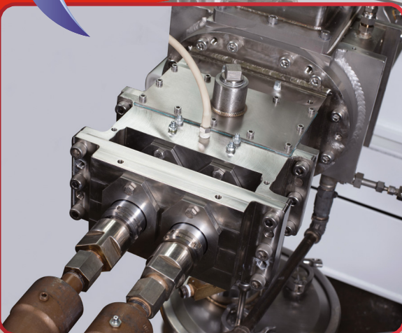
High temp rotary couplings for continuous heating or cooling media through rotating shafts.
