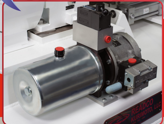
Air over oil actuator to assist in cleaning and changing shafts. Powered by customer supplied compressed air.
