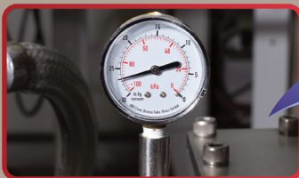
Actual gauge in operation. Over 27" Hg indicated.
