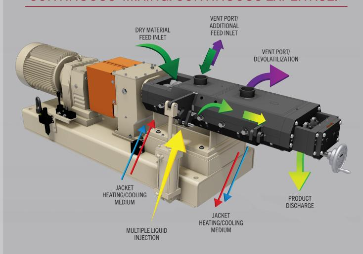
Highly flexible and sturdy, the twin-screw design of Readco's Continuous Processor mixes, processes, and chemically reacts, giving a consistent mix for even the most difficult applications, ensuring consistent and repeatable performance. The Continuous Processor is ideally suited for operations involving reaction, polymerization, crystallization, compounding and heating or cooling of materials up to many million centipoise viscosity.
